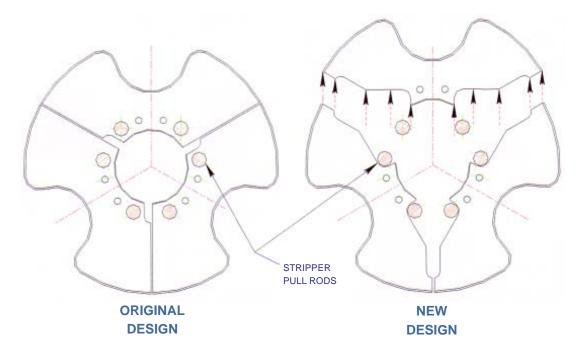
The new design provides clearance cutouts allowing the starwheel segments to be readily removed without disassembly from the stripper pull rods.
