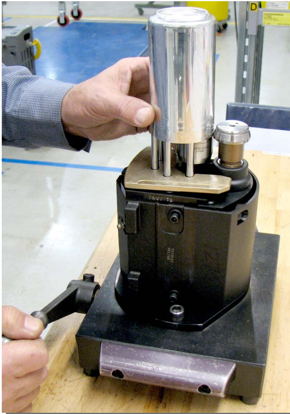
Figure 2. Depth Of Cut Gauge Fixture set up with a CC93 cartridge checking the depth of cut of a can.
