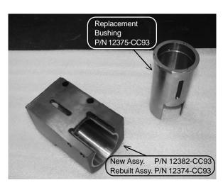
This design will be a standard component as of January 2002, and will be on all new Belvac CC93 and CC95 machines built and shipped after that date.
