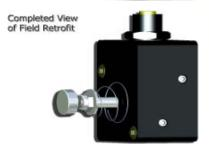
3.) Depress manual override button and rotate ¼ turn to engage manual override locking function. If flat washer comes into contact with black cover and does not allow manual override to lock, remove manual override button, loosen M5 stop nut two turns, reinstall manual override button and re-test.
