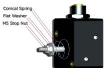
2.) Install conical spring (from upgrade Kit) over extension shaft with larger diameter end of spring located against black cover and small diameter of spring located at thread end of extension shaft. Install flat washer on top of conical spring. Next install M5 stop nut on top of flat washer. Tighten M5 stop nut until it comes to rest against shoulder on manual override extension shaft. Install manual override button on extension shaft and tighten.
