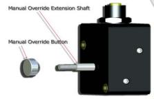
1.) Grasp manual override extension shaft with locking needle nose plier below shaft threads. Grasp manual override button with second set of pliers and gently rotate override button counterclockwise to remove. The button is installed with vibraloc and thread lock, so application of heat may be necessary.
