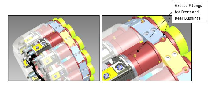
To extend the life of the HyComp bushings and tooling spindle ram, Belvac has provided a manual grease fitting lubrication feature to the Reformer Tooling Cartridge as standard for Reformers issued after September 2017.
