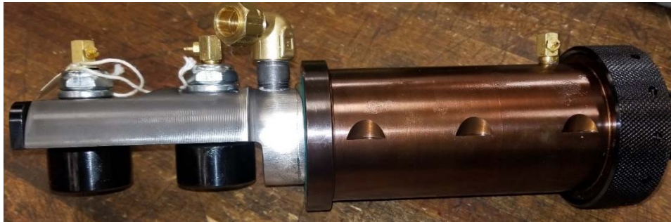
Cam Followers installed on a 595 style ram assembly
