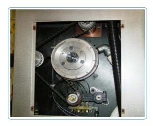
To remove the pulley: release the tensioner, remove the bushing by removing the three screws and jacking the bushing from the pulley.
