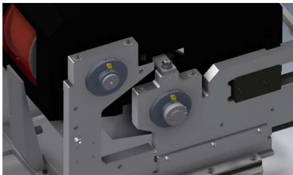
Figure 3: New Side Frame with New Bearings
