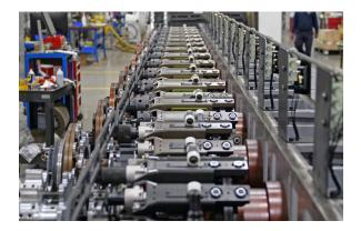
The integral Can Neck Lubrication infeed applies a consistent strip of hot wax or mineral oil on the open end of the can, which occurs without touching the wick. This design removes roller assemblies and the gear drive box resulting in reduced parts, and less maintenance.
